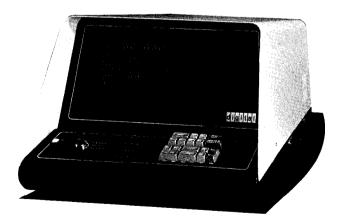
The new controllers supported approximately twice as many digital inputs and outputs using unique single point plug-in signal converters. A significant advantage is the large number of internal logic functions available to the user at no additional cost for timing, counting and shift registers.
