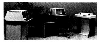
The Datasystem 322 is a floppy diskette based system with 32K bytes of memory packaged in the same desk as the DS310 and using a VT52 CRT. It can be configured with more memory, additional terminals, more mass storage, and a variety of printers.
