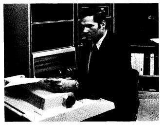
the 11T55—DIGITAL's fastest FORTRAN system. Its 32K bipolar memory, FP11-C floating point option and FORTRAN IV-PLUS will win all computational benchmarks requiring 32K words of memory. Program sizes larger than 32K require the 11/70 for optimum performance due to the 32K bipolar memory limit on the 11/55.
