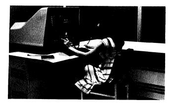
a superset of the VT11 instruction set. The GT62 is a terminal configuration based on the VS60 and a PDP-11/10. With the introduction of the 11/34, the GT62 received a CPU upgrade making the GT62 an even more powerful graphics terminal.
