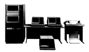
The Datasystem 324, also using an LSI-11, is an RK05 disk based system. Offered in the new Datasystem cabinets, the basic system consists of 32K bytes of memory, a VT52, and an RK05J and RK05F. It, too, can have more memory, more terminals, more mass storage, and a variety of printers.
