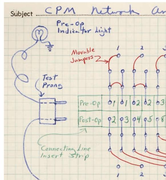
analogy of a project schedule. The Indicator Circuit was used to probe the plugboard, entries were made into a worksheet, and the schedule was then manually recalculated. With the help of Stanford's Electronics Lab, Fondahl constructed the more sophisticated Project Network Analyzer in 1964.
