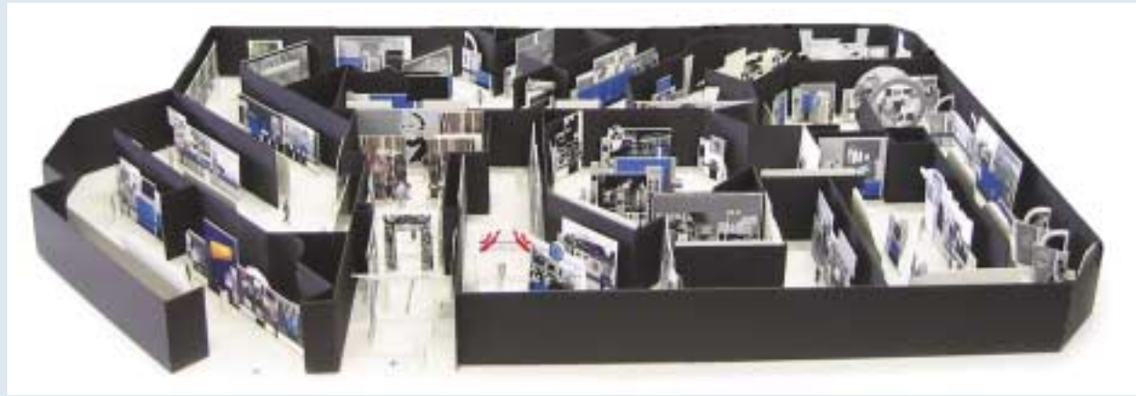
To understand how much space will be required for an exhibition and determine the best adjacencies of exhibit areas, exhibit designers create space study models such as the one shown here.
