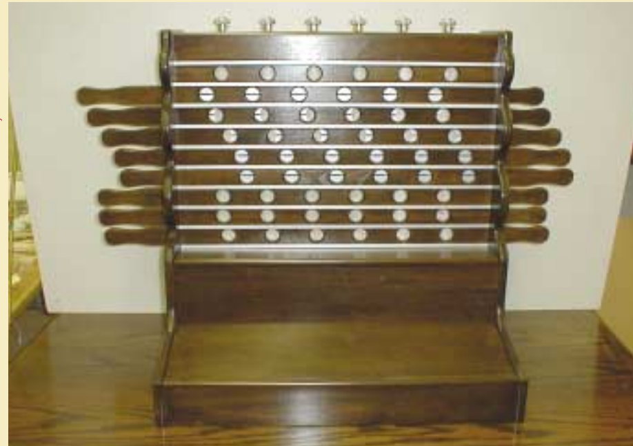
First prototype Schickard Rechenmaschine in the workshop at the Museum of Science.
