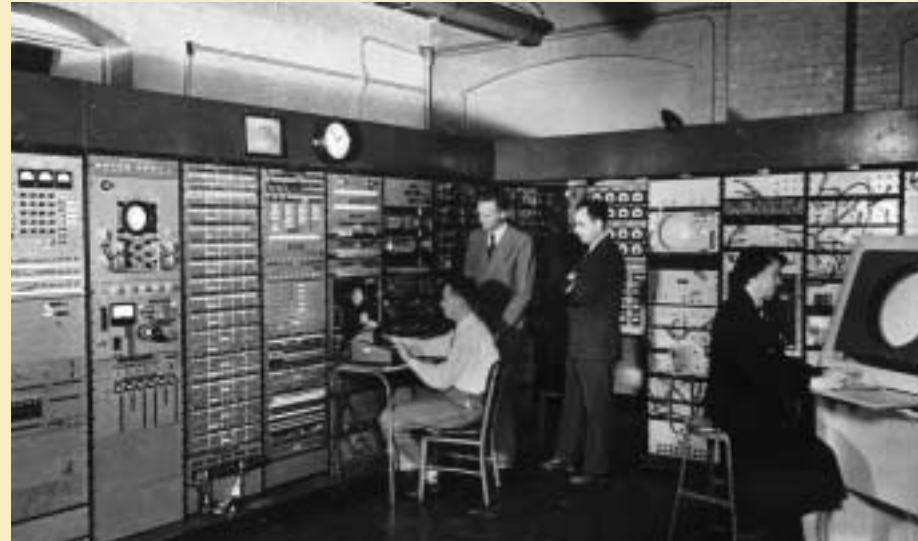
Whirlwind was the first real-time, parallel-processing computer with core memory. At left are the marginal checking and toggle-switch test control panels. From left to right: Stephen H. Dodd, Jay W. Forrester, Robert R. Everett, and Ramona Ferenz, 1951.
