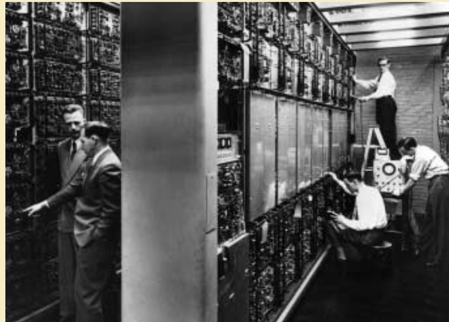
The internal workings of Whirlwind. Here, the machine's size dwarfs three technicians (John A. O'Brien, Charles L. Corderman, and Norman H. Daggert) working on the Electrostatic Storage Rack. At left, Jay Forrester and Norman H. Taylor inspect the Arithmetic Element Rack, 1952.
