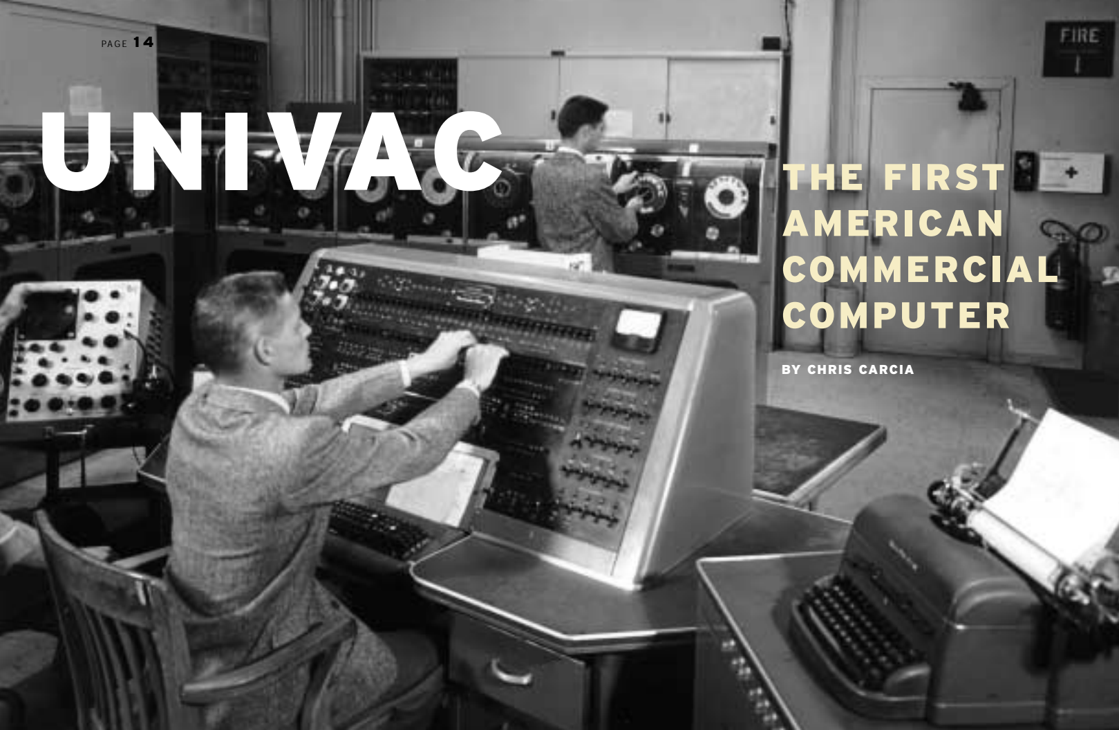
Operator (front) at the UNIVAC console while colleague mounts a new data tape on a UNISERVO tape drive.
