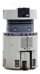
detect anything within a 150-foot radius and send back a message if anything unusual was detected. The robot could patrol for up to 14 hours at a time, and could return itself for charging when necessary. Denning intended the sentries to patrol a variety of facilities from prisons to factories.\*
