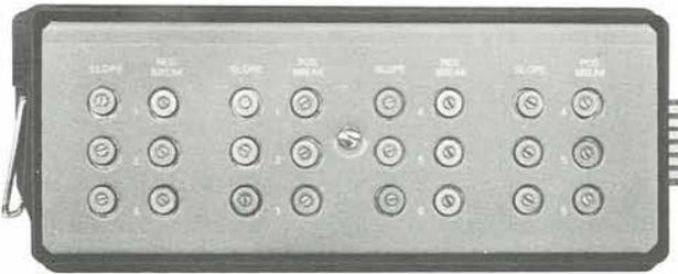
**Fixed Function Cards:** The 3351 VDFG (shown) and the high-resolution 3352 VDFG can be supplied with fixed functions, e.g., sine  $\pm 90^\circ$ , cosine  $\pm 90^\circ$ , Log |X| (range of X 1 to 100 volts). Each VDFG channel is terminated on the patchboard on Models 3321, 3322, and 3325.
