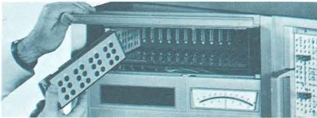
**SD 40/80:** Built-in provision for 15 Model 3351 or 10 Model 3352 high-resolution VDFG cards. Functions are set up with the help of a Model 3341 FG Set-up Unit which brings the VDFG card out into the open for easy screwdriver pot adjustment of breakpoint and slope.
