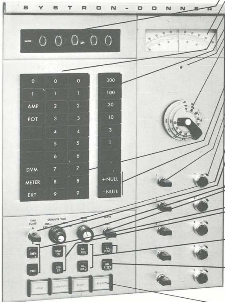
Function Generator Receptacle holds up to 15 Model 3351 (or 10 Model 3352 high resolution) V.D.F.G. plug-in cards.
