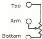
All other groups are 2-terminal with the bottom of the potentiometer internally grounded. The input voltage to the potentiometer is applied to the top terminal and the output is available at the arm terminal.
