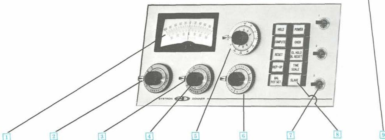
**1 Meter Readout Ranges:** 1, 3, 10, 30, 100, and 300 volts, and  $\pm$  null. Full scale accuracy: 3%. Null position provides 0.02% F.S. resolution with reference potentiometer having a  $\pm 0.05\%$  linearity at 25°C.
