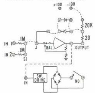
(CONNECTIONS SHOWN FOR COMPARATOR AMPLIFIER.)
