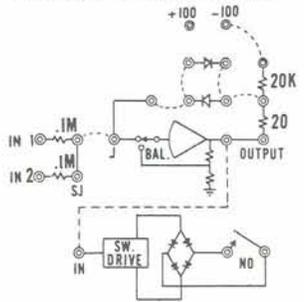
(CONNECTIONS SHOWN FOR COMPARATOR AMPLIFIER.)
