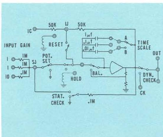
Feedback Capacitors (in oven) 1  $\mu$ F, 0.1  $\mu$ F: Trimmable to better than 0.01%.
