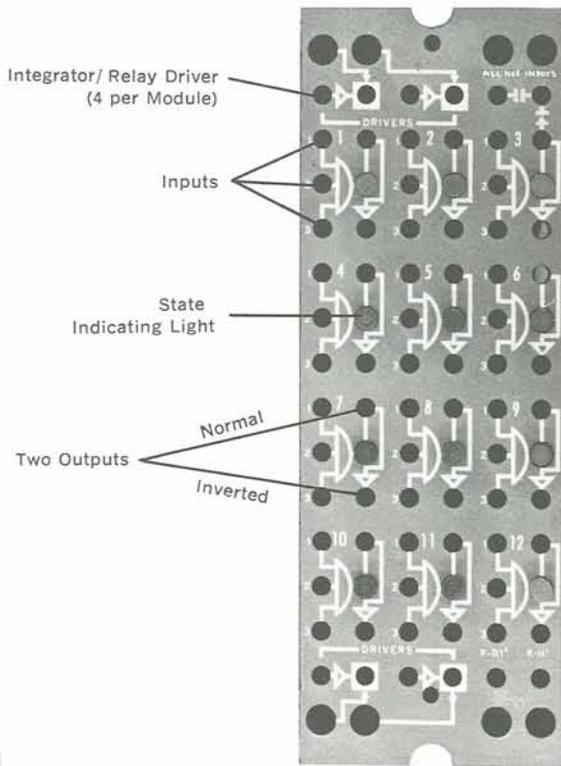
The Model 3327 contains 12 identical AND gates and four relay drivers. Each gate has three input terminals, two output terminals and a state indicating lamp.
