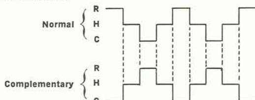
Figure 1. Mode Duty Cycle for Integrators in Iterative Operation
