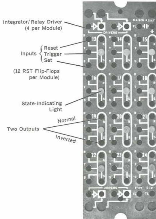
The flip-flop module contains 12 identical RST flip-flops and four relay drivers. Five patchboard terminals are available for each flip-flop, plus a state indicating lamp.
