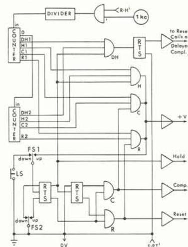
Figure 2. Iterative Operation Logic Control Circuit
