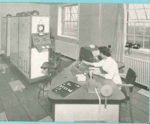
The 'basic' Zebra, shown above, is used mainly for mathematical and scientific research. Because it can be adapted for use with most forms of input/output equipment, Zebra can also serve as the control centre for small or medium-sized Data Processing Systems.
