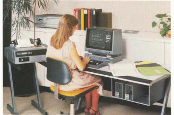
Approximately 135,600 bytes of disk storage space from the two mini-disk systems. Tractor feed line printer uses fanfold paper with feed holes in the margins and will produce up to 5 carbon copies. The System Desk has recessed spaces for the Expansion Interface and keyboard with interconnecting wiring concealed. Line printer stand leaves more desk space.
