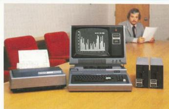
Two mini-disk units give user approximately 135,600 bytes of disk storage. Virtually all TRS-80 disk-based business software requires this as a minimum system. Applications include general ledger, payroll, disk mail list and more. Line Printer II adds real versatility and convenience to this system, without taking up a lot of work space.
