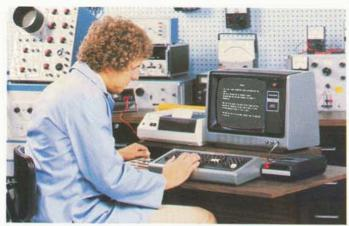
For more technical applications, the "Engineer" system combines powerful Level II with 16K of RAM. The new Printer Interface cable allows direct connection of the Quick Printer to TRS-80's bus connection, without using the Expansion Interface. Quick Printer provides 80-column hard copy and program listings. The Space-Saver holds the entire system and provides the user with ample work space.
