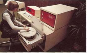
QANTEL Model 3001 Disc Drive provides six million characters of data storage: three million removable for offline storage, and three million for fixed information. Model 3101 provides 12 million characters of data storage,
