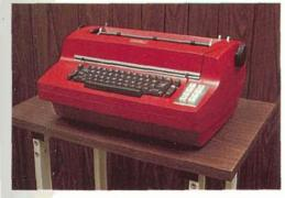
QANTEL Model 4201 Selectric Terminal transmits data to and receives data from the computer, typing out data at 15 characters per second.
