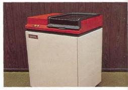
QANTEL Model 3201 Disc Drive provides 30 million characters of quickly accessible data storage. Four Model 3201 Disc Drives can be supported by Systems 1100 and 1200, giving up to 120 million characters of disc storage.
