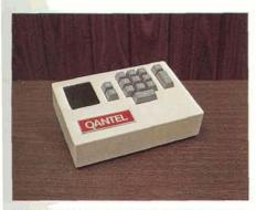
QANTEL's 10-key console is a desk-top device with an adding machine keyboard configuration, used for entry of numeric data only.
