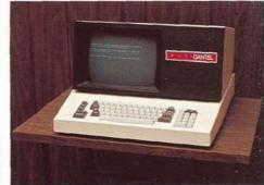
QANTEL's Model 4011 Video Terminal has all the features of the 4001 Video Terminal plus a large, 1728-character screen. The Video Terminals all have the capability of communicating with the computer via telephone lines.
