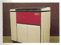
Models 5021 and 5031 are both variable speed line printers, functionally different only in their high rates of printing speed. Model 5021 can print 245 to 1100 lines per minute, and 5031 can output at 700 to 1800 lines per minute.
