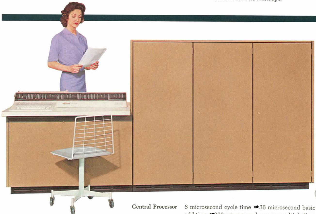
Central Processor 6 microsecond cycle time • 36 microsecond basic add time • 900 microsecond average multiply time
