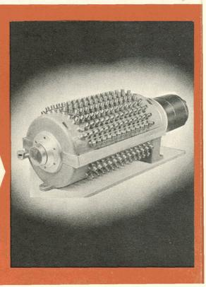
Intelligence is recorded on the drum as combinations of magnetized marks or spots. Information thus recorded is represented by combinations of two possible states of the medium (binary representation)—a technique commonly used with relays, punched tape, and punched cards. Combinations of marks can represent decimal numbers, characters of the alphabet, or other forms of intelligence.
