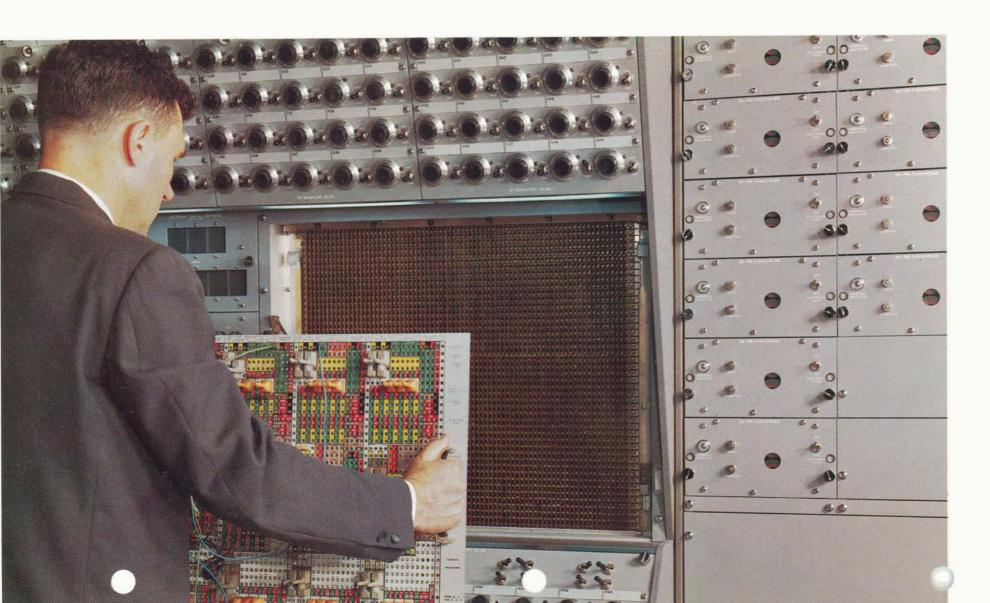
The exceptionally high accuracy of the *Pace 231R* Computer stems from the newly developed d-c amplifier package. Each position contains four independent, extremely low drift d-c amplifiers, which provide high linearity over a wide band width.
