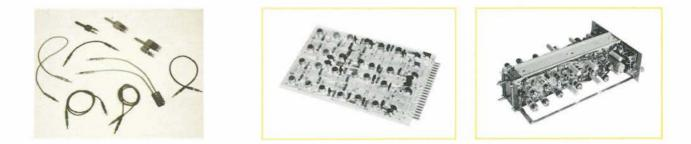
All components are plug-in, drawer type units which feature miniaturization and printed circuitry to keep maintenance to a minimum.
