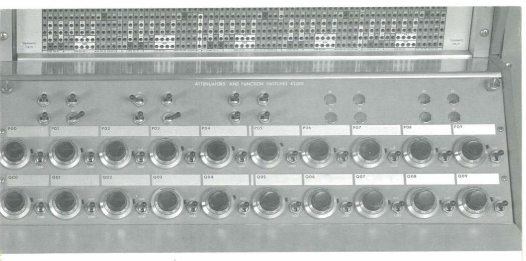
*Human Engineered Control Panel* contributes to faster, more accurate problem solving. Push buttons and switches are laid out in individual sections according to the operation they serve. Panel is inclined to put all controls within easy reach and view of operator.
