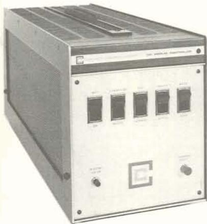
The CC-301 TV Display Controller is the heart of both the CC-30 and CC-33 stations. It displays alphanumeric or graphic data on a standard television receiver (a big factor in keeping the cost of the station far below others), accepts information from a keyboard or other input device, controls all input/output devices at the station, and communicates with any computer.
