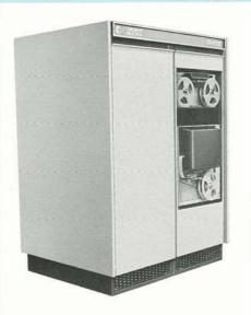
The auxiliary cabinet of the CIP/4000 which contains the I/O module, the tape reader, and the DRPE punch.
